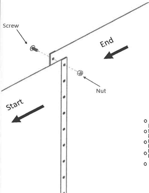
Begin inserting the wall into the bottom wall tracks in the middle of a joiner plate. At first, the wall should be kept in place with one or two support bars (or extra persons). One person should uncoil the wall on a beam or a plank while a second person inserts it in the bottom wall tracks. Do not uncoil more than 3 m (10') of wall before you install a support bar to reinforce the structure.
