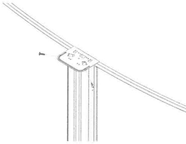
Install the joiner plates on top of each upright then install metal screws at the top of the support posts, making sure the support posts are perpendicular to the ground.
