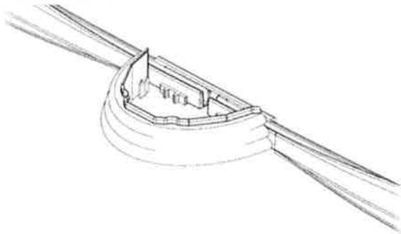
Assemble all bottom tracks to the bottom plates to form a perfect circle with a diameter and a radius in accordance to the chart
